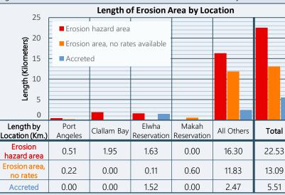
A total of 35.6 kilometers of erosion areas were found. Within the erosion hazard areas, the maximum retreat rate was 8.8 m/yr east of the Elwha River mouth and the average retreat rate was 0.9 m/yr (median = 0.4 m/yr). Over 13 kilometers need additional data sources to better understand the magnitude of erosion.
