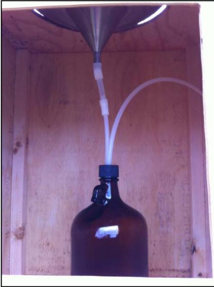
Drainage tubing from funnel to sample bottle, and air vent.
